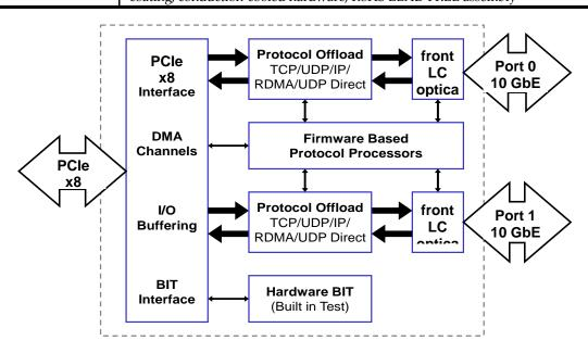
**Block Diagram:** Functional block diagram for the XGE4120 CCXMC by Critical I/O. This CCXMC provides two independent 10 Gb Ethernet ports, each with integrated protocol offload hardware. Dedicated hardware offload provides full duplex operation at wire-speed, up to 2500 MB/s (2.5 GB/s) (per port).
