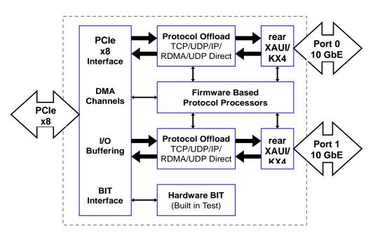
**Block Diagram:** Functional block diagram for the XGE4120 CCXMC by Critical I/O. This CCXMC provides two independent 10 Gb Ethernet ports, each with integrated protocol offload hardware. Dedicated hardware offload provides full duplex operation at wire-speed, up to 2500 MB/s (2.5 GB/s) (per port).
