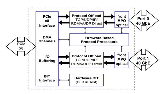
**Block Diagram:** Functional block diagram for the XGE4423 CCXMC by Critical I/O. This CCXMC provides dual independent 40 Gb Ethernet ports, each with integrated protocol offload hardware. Dedicated hardware offload provides full duplex operation at wire-speed,up to 10 GB/s (per port).
