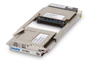
StorePak combines a removable storage module with a fixed carrier base module
