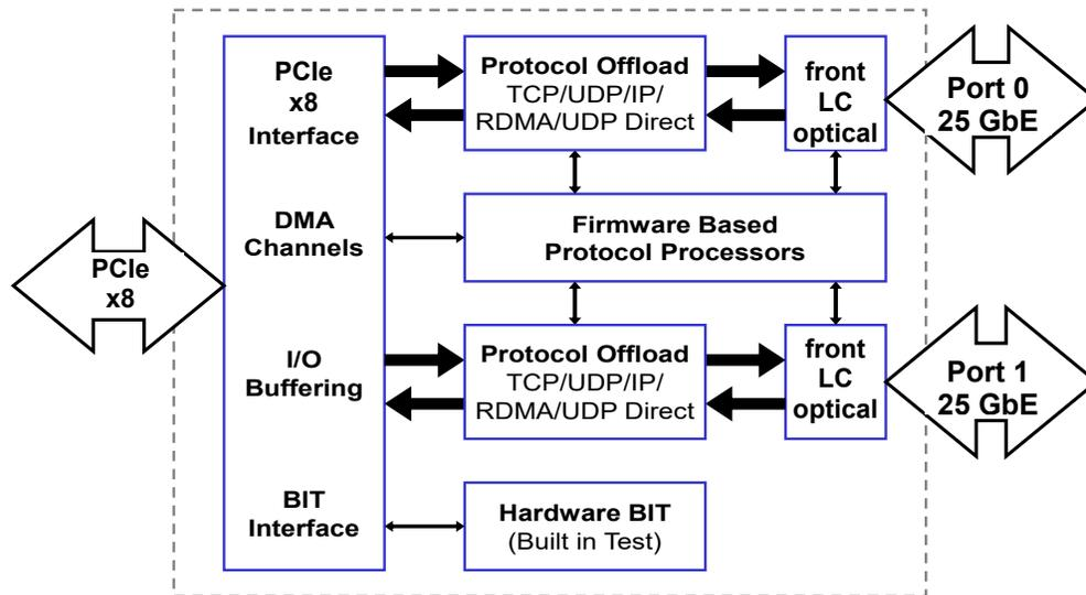
**Block Diagram:** Functional block diagram for the XGE4224 CCXMC by Critical I/O. This CCXMC provides dual independent 25 Gb Ethernet ports, each with integrated protocol offload hardware. Dedicated hardware offload provides full duplex operation at wire-speed, up to 6.25 GB/s (per port).
