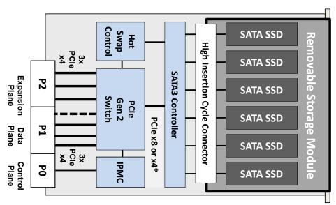
Dashed PCIe x4 connection is present in SC300 version only \* PCIe x4 in SC300 version, PCIe x8 in SC300P version
